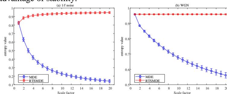
Fig.2. The comparisons of MDE and RTSMDE for WGN and 1/f noise: (a) analysis results of 1/f noise, (b) analysis results of WGN.
