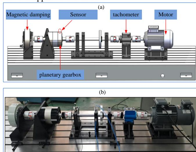
Fig.3. The experimental planetary gearbox system: (a) the layout of the test rig, (b) the test rig.
