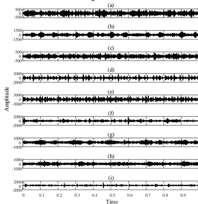
Fig.5. The time-domain waveforms of vibration signals: (a) healthy gear, (b) sun gear with a spalling tooth (SGST), (c) sun gear with a cracked tooth (SGCT), (d) sun gear with a broken tooth (SGBT), (e) sun gear with a missing tooth (PGMT), (f) planet gear with a broken tooth (PGBT), (g) fracture of bearing cage (FBC), (h) planet gear with a spalling tooth (PGST), (i) planet gear with a missing tooth (PGMT).
