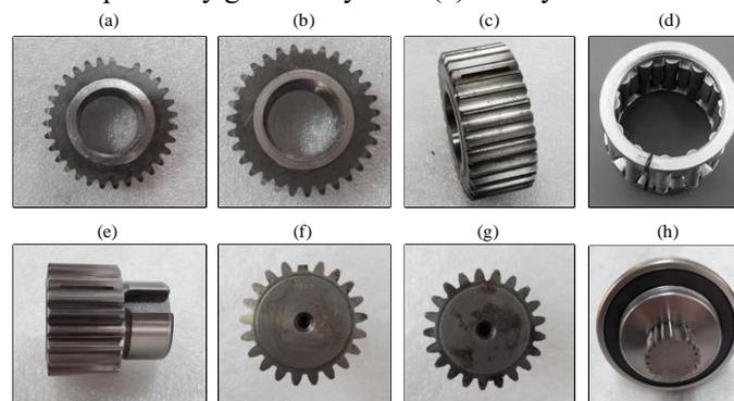
Fig.4. (a) planet gear with a missing tooth (PGMT), (b) planet gear with a broken tooth (PGBT), (c) planet gear with a spalling tooth (PGST), (d) fracture of bearing cage (FBC), (e) sun gear with a spalling tooth (SGST), (f) sun gear with a broken tooth (SGBT), (g) sun gear with a cracked tooth (SGCT), (h) sun gear with a missing tooth (PGMT).
