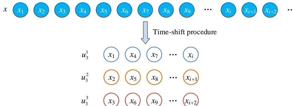
Fig.1. The illustration of time-shift multiscale analysis with  $\alpha = 3$ .
